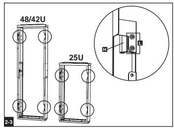
With the aid of an assistant, lift the frame, align the frame's hinge swivels with the rack enclosure's hinges and hang the frame from the hinges. When the frame is securely aligned with the rack enclosure, tighten the hinge swivel screws that you loosened in the previous step.
